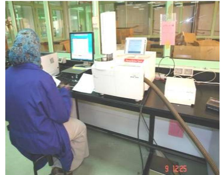
*Differential Scanning Calorimeter (DSC)*
