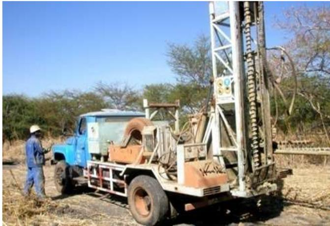
**Dongfeng auger rig Drilling Shot hole**
