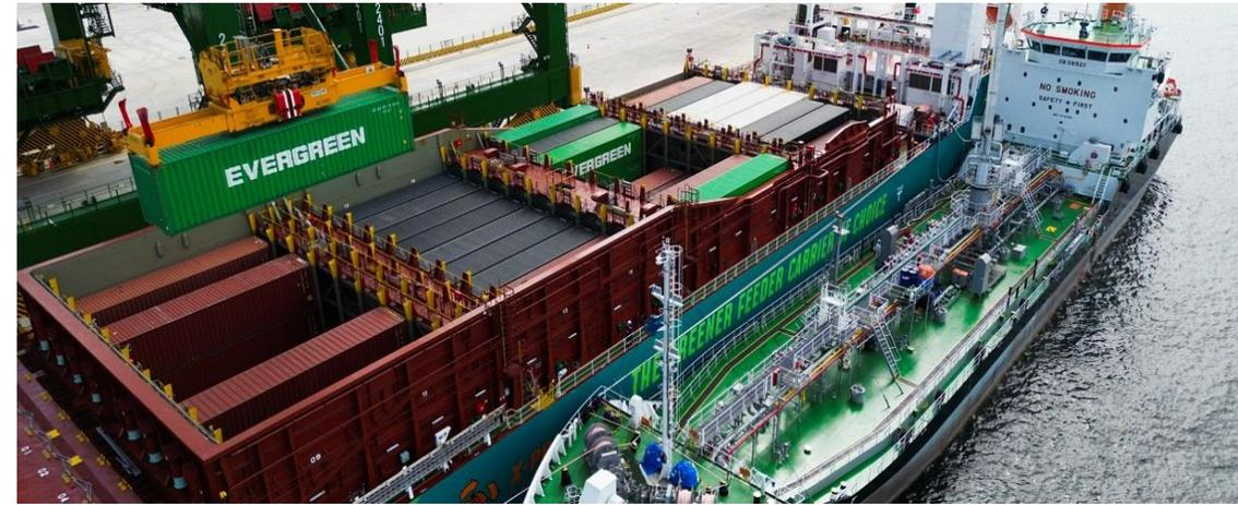
*First simultaneous methanol bunkering and cargo operation*
