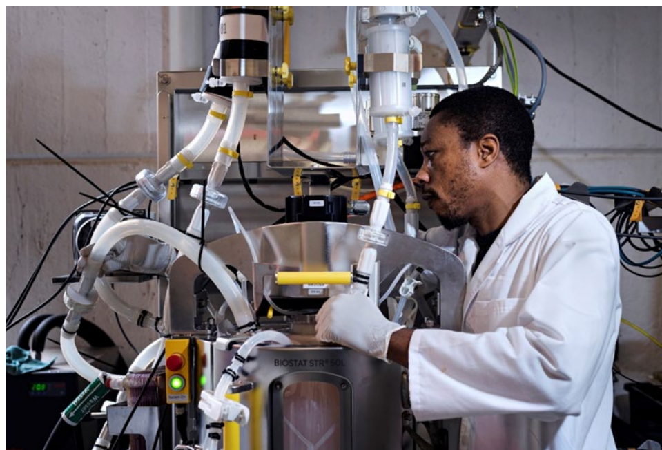
Seaweed fermentation to produce PHAs. Credits: Uluu, 2024
